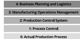
Figure 1. Functional hierarchy model for a manufacturing enterprise, depicting the five hierarchy levels (Level 0 – Level 4) in industrial automation [1].
